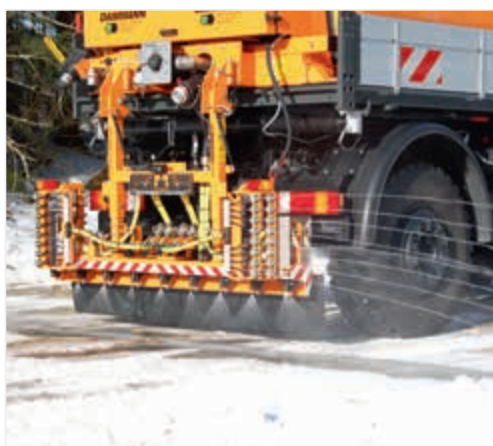
De-icing of traffic areas (e.g. airports, roads) with saline solution is an effective and economical process. Here, low-drift ID nozzles are used in combination with VarioSelect® for variable nozzle control in order to maintain a constant application quantity at changing driving speeds.
