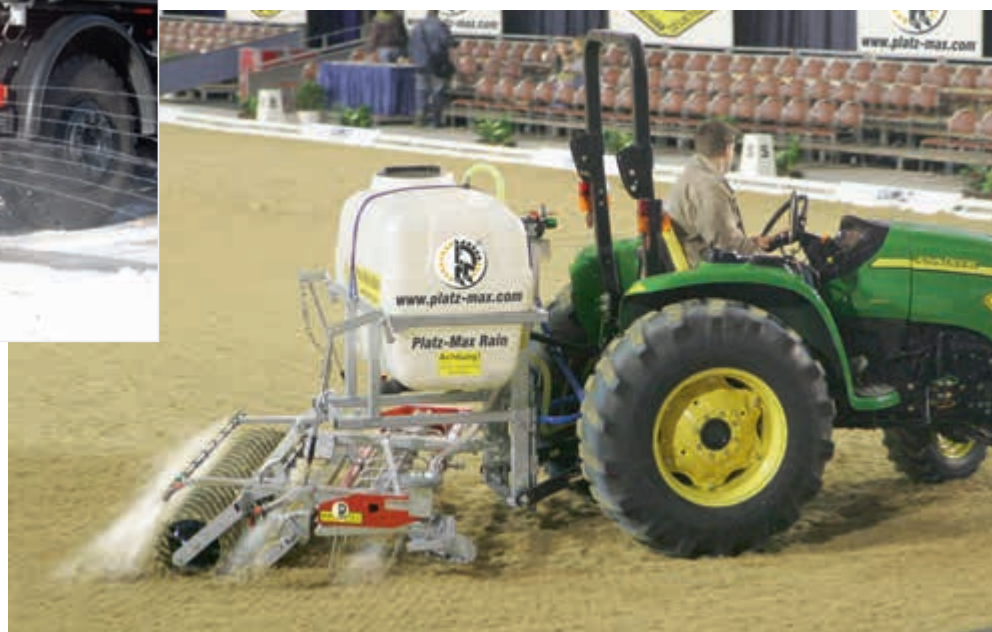
Riding arena watering. A total of 3 nozzle rows equipped with the ID air-injector nozzle ensure an optimally watered arena floor in combination with a rake, tilling roller and smoothing attachment.
