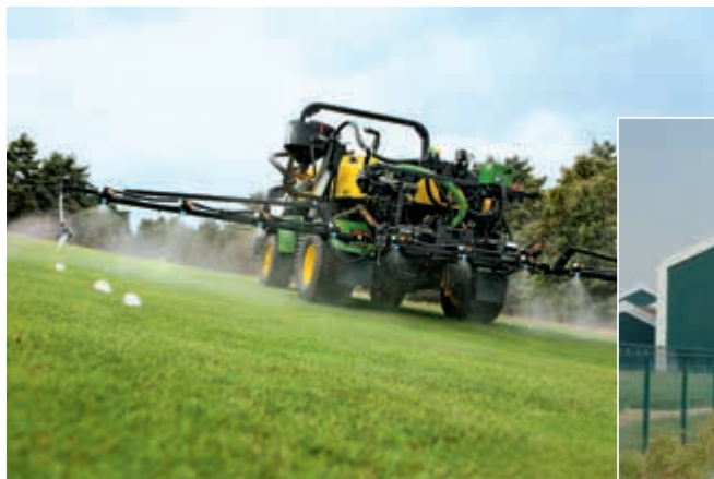
Low-drift application on golf courses with air-injector flat spray nozzles ID, IDK, IDTA and IDKT
