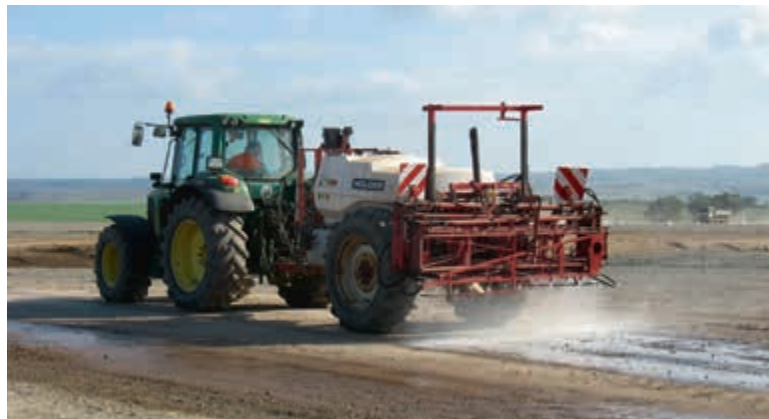
Dust binding on traffic areas with ID and FD nozzles Source: RAW Handel und Beratungs GmbH
